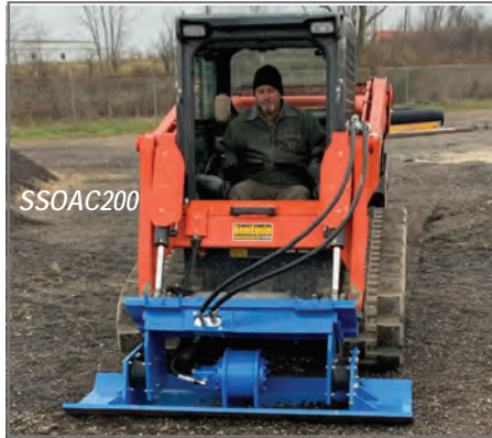
72" wide tamper base plate, suitable for skid steer loaders.
