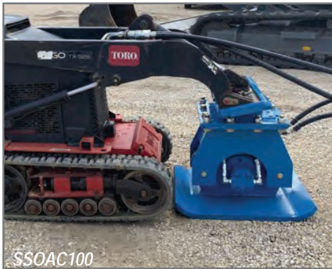
24" wide tamper base plate, suitable for compact utility loaders.
